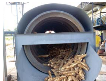
Figure 1 A Trommel-type cassava cleaning machine
