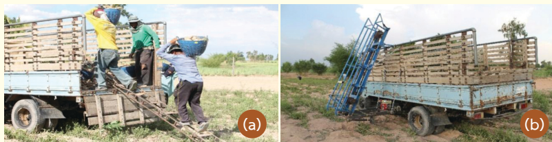
Figure 1 Show methods of cassava collection from field a) conventional b) equipped with conveyor mounted to harvesting truck
