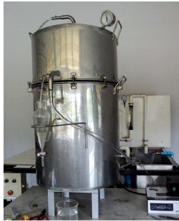
Figure 1 Distiller for the small industry or community level
