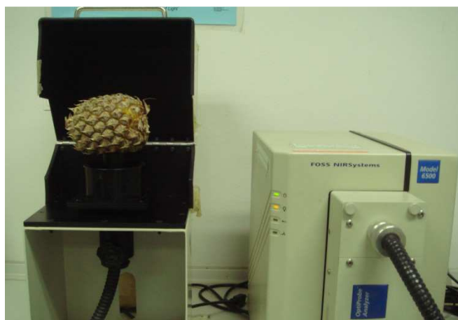
Figure 1 Measurement of pineapple fruit spectrum using NIRSystem 6500 with fiber optic probe
