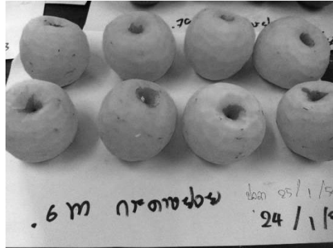
Figure 2 Evaluating the bruised area of apples by peeling.
