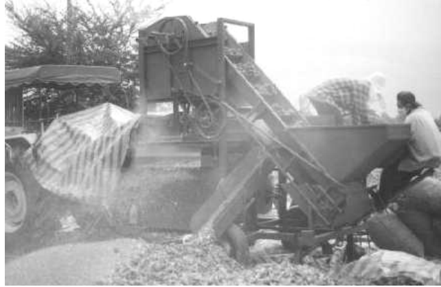
Figure 1 Sunflower thresher during operation.
