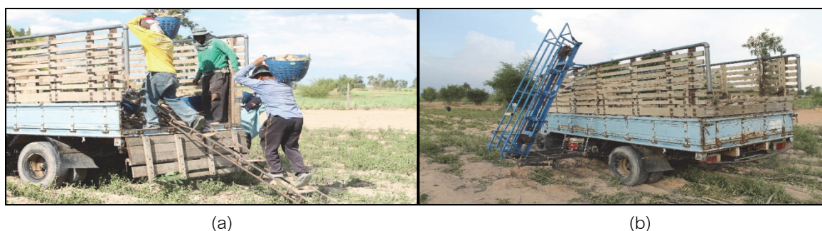
Figure 1 Show methods of cassava collection from field a) conventional b) equipped with conveyor mounted to harvesting truck
