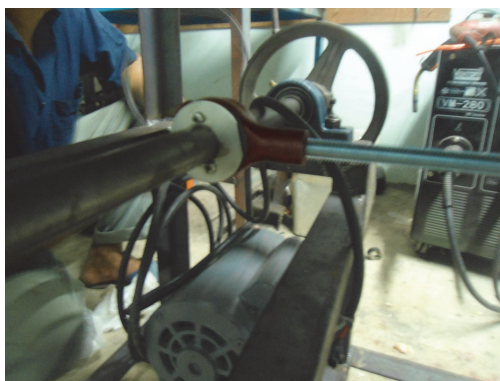
Figure 2 Rotating shaft with a 5mm eccentric coupling
