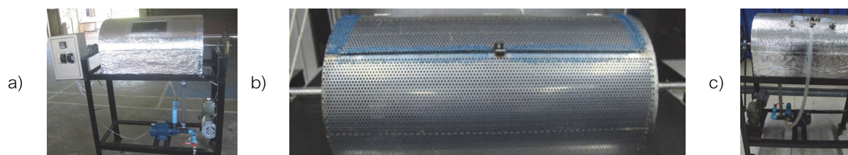
Figure 1 a) Paddy germination machine (PGM) b) sieve bin and c) nozzles locations
