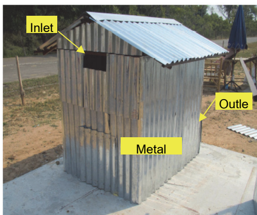
Figure 1 Experimental set up of greenhouse solar dryer with triangle roof type
