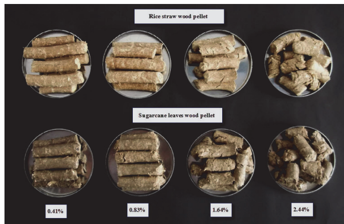
Figure 4 Rice straw for biomass fuel pellet and sugarcane leaves pellet
