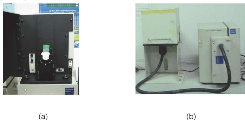
Figure 2 NIRSystem 6500 with (a) transportation module and (b) fiber optic with interactance probe
