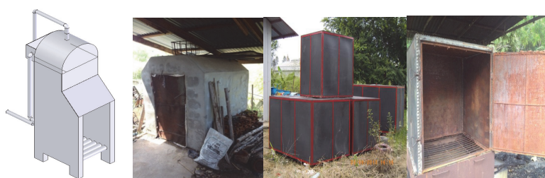
Figure 1 a) Steam Boiler b) chamber with brick wall c) chamber with synthetic rubber wall d) chamber with steel wall.
