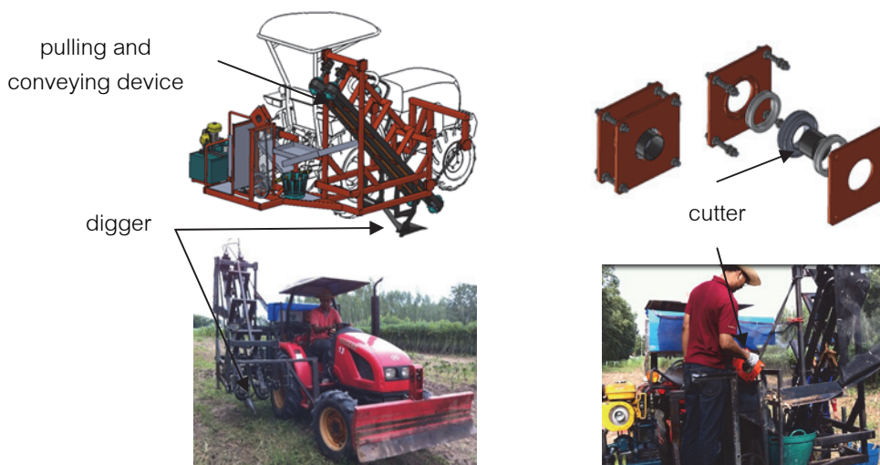
Figure 1 A developed cassava harvester for cutting cassava tuber from rhizome
