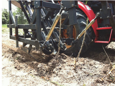
Figure 3 Cassava harvesting using the developed harvester
