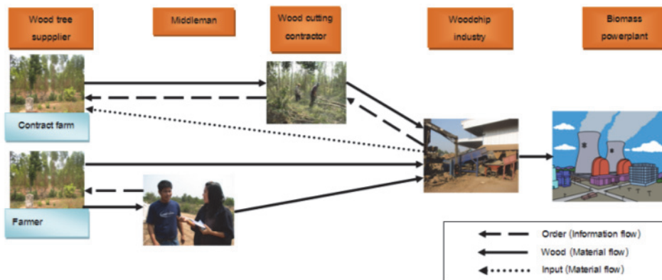
Figure 1 Logistics structure of wood supply chain to biomass power plant
