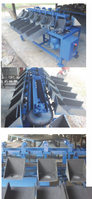
Figure 2 The prototype of sugar apple sizing machine
