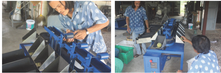
Figure 3 Testing sugar apple sizing with the prototype machine
