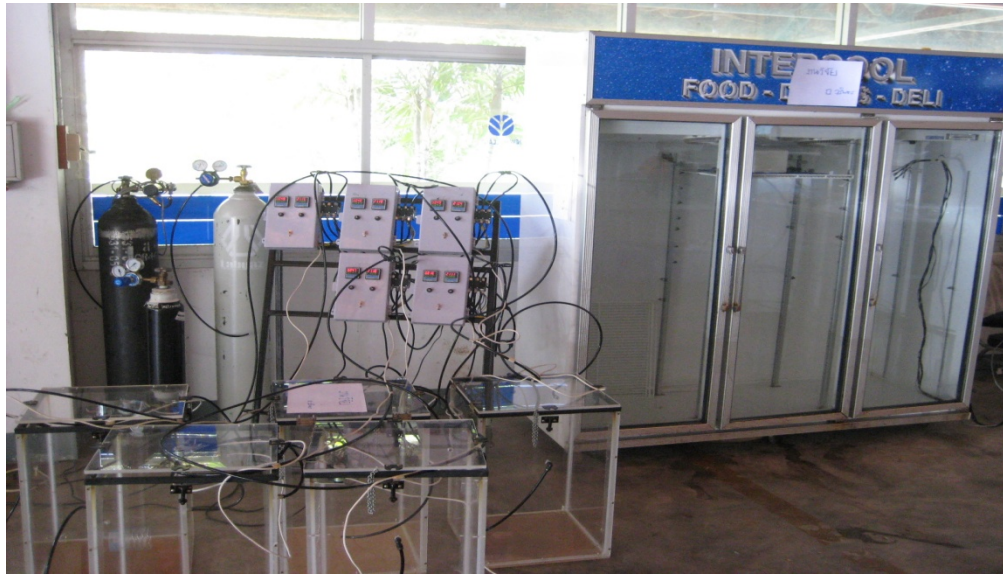
Figure 1 Controlled atmosphere storage system of agricultural produce for retailers
