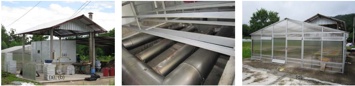
Figure 2 The improved flesh longan drying plant having additional solar energy from greenhouse effect; (a) improved furnace, (b) improved drying room, (c) improved heat exchanger, (d) additional solar greenhouse
