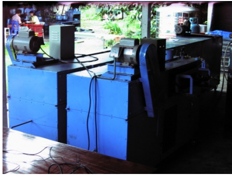
Figure 6 Continuous Type Longan Dryer
