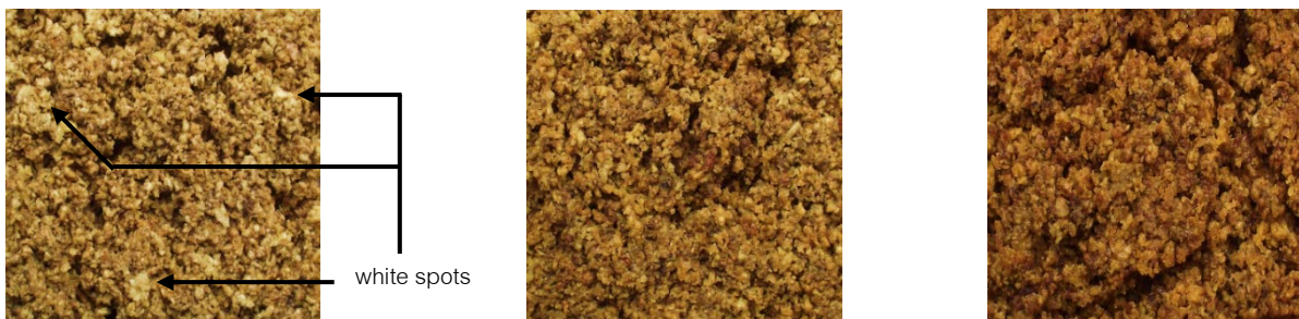
Figure 3 Show physical quality after drying block rubber STR 20 by hot air-microwave; (a) at 100°C, drying times < 6,400 seconds (b) at 100°C, optimal drying times 6,400-8,000 seconds and (c) at 120°C, drying times > 4,800 seconds
