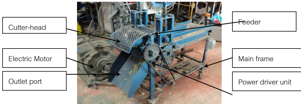
Figure 1 Cane leaf chopping unit
