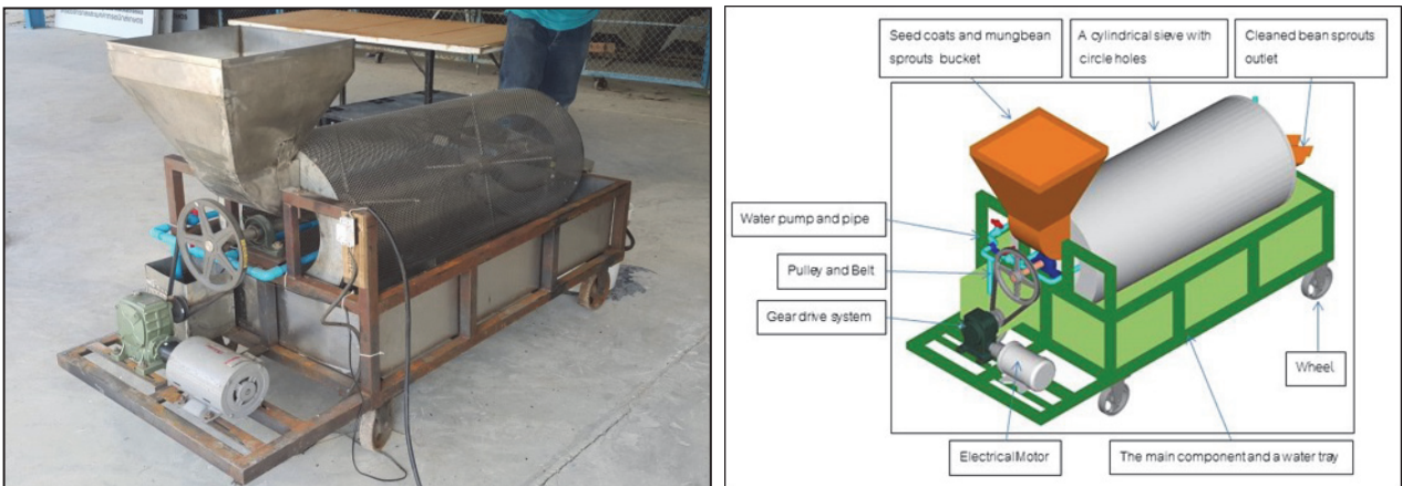
Figure 1 Components of a seed coat separator and cleaner for mungbean sprouts (germinated black mungbean seeds)
