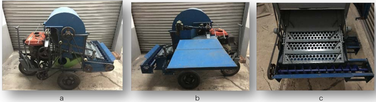
Figure 2 (a) Groundnut Stripping Machine (b) Feeding Tray (c) Sieve and Screw Convey
