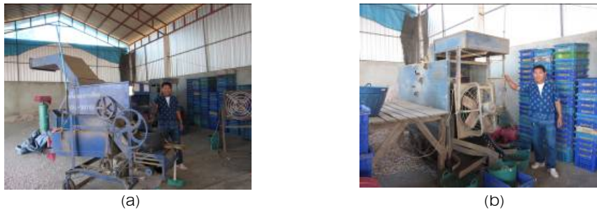
Figure 1 The commercial garlic sheller; (a) one rod of cylindrical rubber roller. (b) three rod of cylindrical rubber roller
