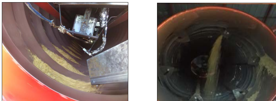
Figure 2 Drying Germinated Brown Rice by rotary dryer using infrared ray combined exhausted hot air.
