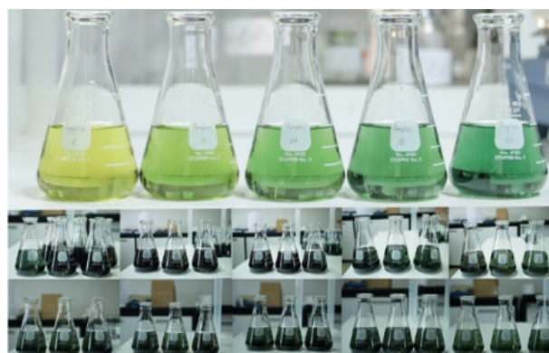
Figure 2 Value and Color of standard amylose content comparison with 10 Japanese rice samples.
