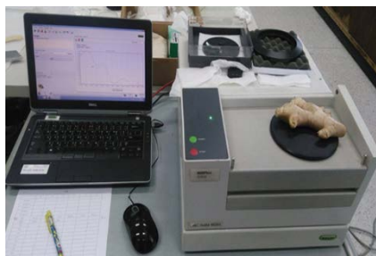
Figure 2 Measuring the spectra by NIR Flex N-500
