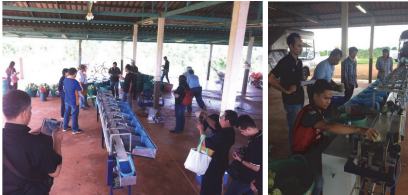
Figure 4 Testing sugar apple sizing with the prototype machine
