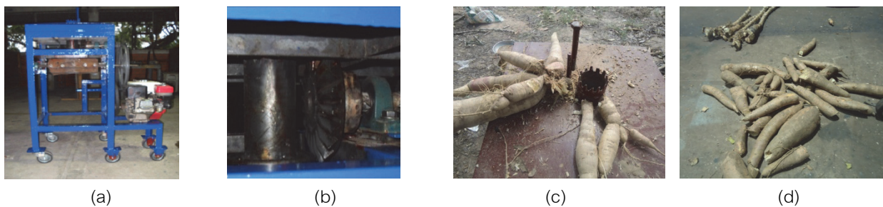
Figure 4 Cassava tuber cutting machine depart cassava rhizome
