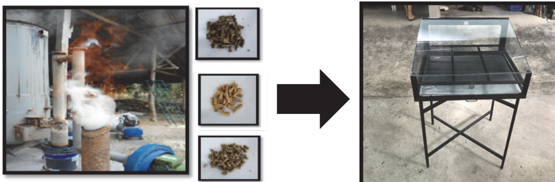
Figure 2 The construct of solar downdraft gasifier with rice husk as fuel dryer
