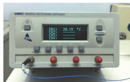
Figure 6 Fiber Optic Thermometer
