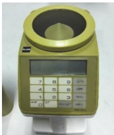
Figure 3 Moisture Content Meter
