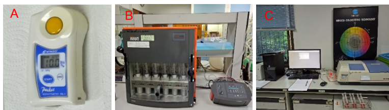
Figure 2 Chemical property analysis of Japanese pumpkin; TSS (A), lipid (B) and starch (C)
