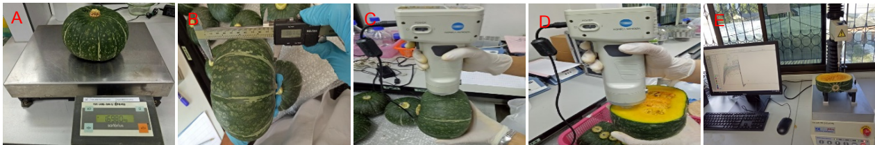
Figure 1 Physical property measurement of Japanese pumpkin; weight (A), dimension (B), peel color (C), flesh color (D) and firmness (E)
