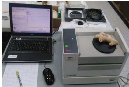
Figure 6 Measuring the spectra by NIR Flex N-500
