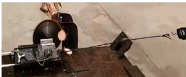
Figure 1 Test the cutting linear speed of the circular saw.
