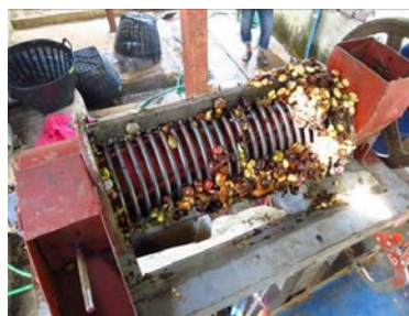
Figure 2 Green cherry coffee separator with vertical housing
