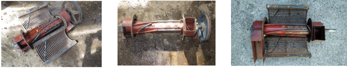
Figure 3 Type 1: Roller unit with teeth and reverse end thread (left) Type 2: Roller unit without teeth but with reverse end thread (center) Type 3: Roller unit without teeth and without reverse end thread (right)
