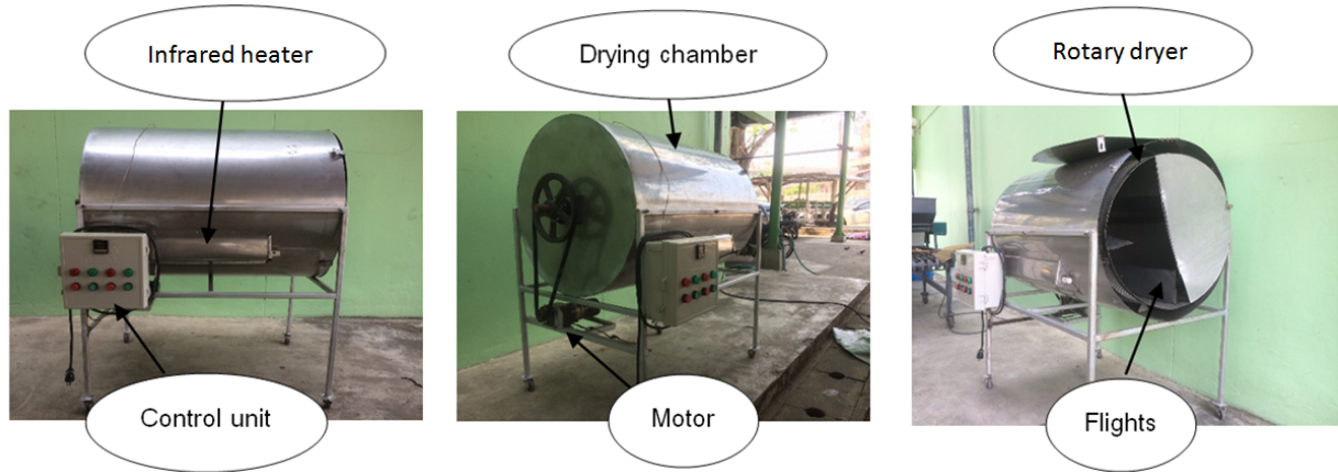
Figure 1 Infrared rotary chili dryer
