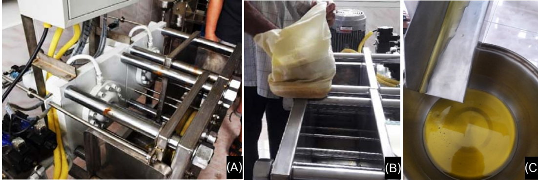
Figure 2 Soybean oil compression testing process with hydraulic compression machine.
