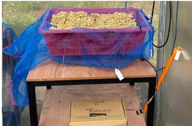
Figure 1 Automatic data logging scales
