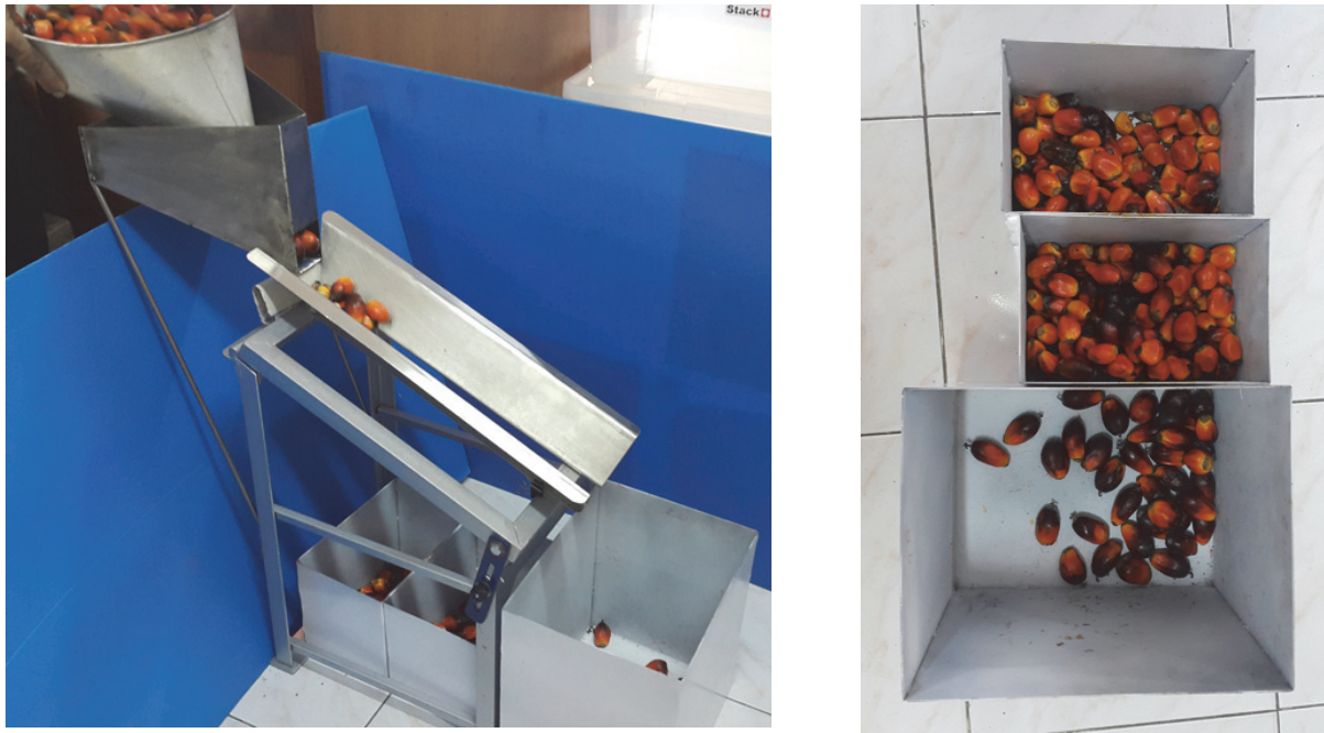
Figure 1 Palm fruit size sorting equipment experiment
