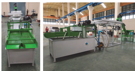
Figure 4. Prototype of arabica cherry coffee cleaning machine for farmer
