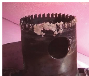
a. Remaining starch stuck on the saw-tooth blade after the cutting
