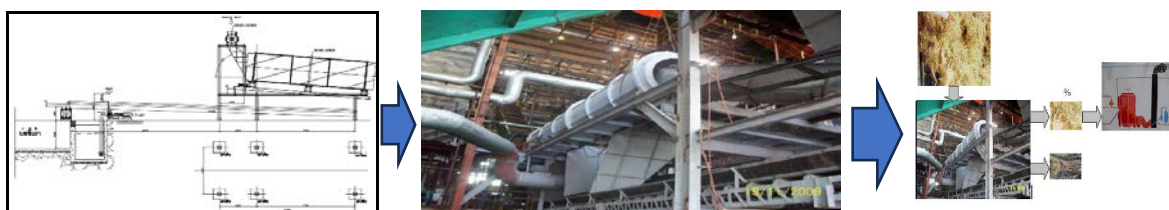
Figure 4 Separating contaminants from bagasse fuel of sugar mills
