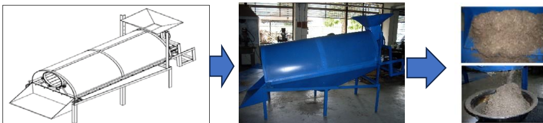
Figure 3 Simulation of a prototype separating impurities from bagasse fuel.
