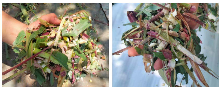
Figure 3 Resulted of the maize shredder machine with different of blade type: smooth edge (left) and serrated edge (right)
