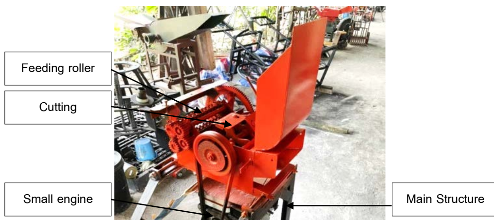
Figure 1 Components of the prototype of maize shredder
