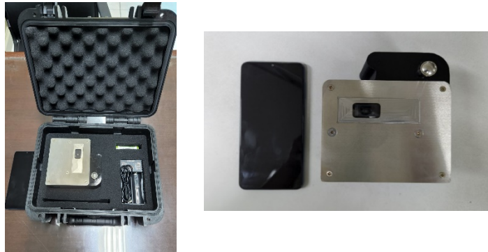
Figure 2 Physical characteristics of near infrared portable amylose analyzer
