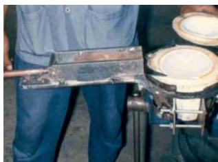
Fig. 2 Shearing of a trimmed young coconut fruit (ycf)
