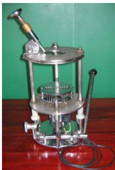
Fig. 7 Developed ycf opening machine (shearing mechanism)
