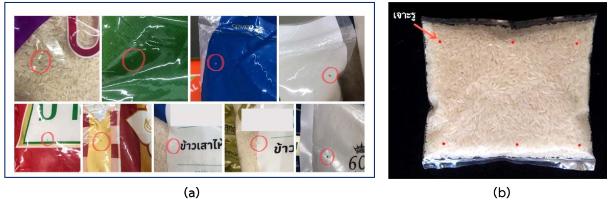
Figure 1. The punched holes with 1 mm diameter presented in milled rice packaging (a) the red dots represented the 1mm-punched holes produced in the experiment to examine penetration in milled rice packages by rice moth larvae (b).
