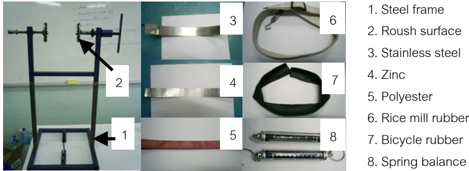
Fig 2 Coefficient friction measuring device of fruits
