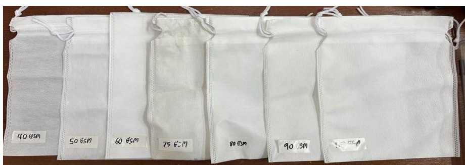
Figure 1 The characteristics of nonwoven spunbonded bags with various densities
