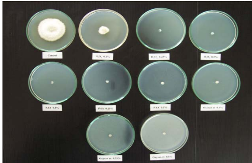
Figure 2 Inhibitory effect of hydrogenperoxide, PAA and Oxyzan® zs at different concentrations on growth of C. gloeosporioides after incubation for 9 days
