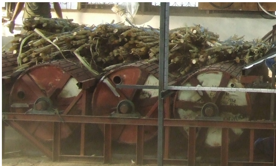
Figure 3 Set of rollers type for separated soil from sugarcane.
